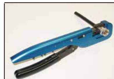
Fold braid over connector and crimp
